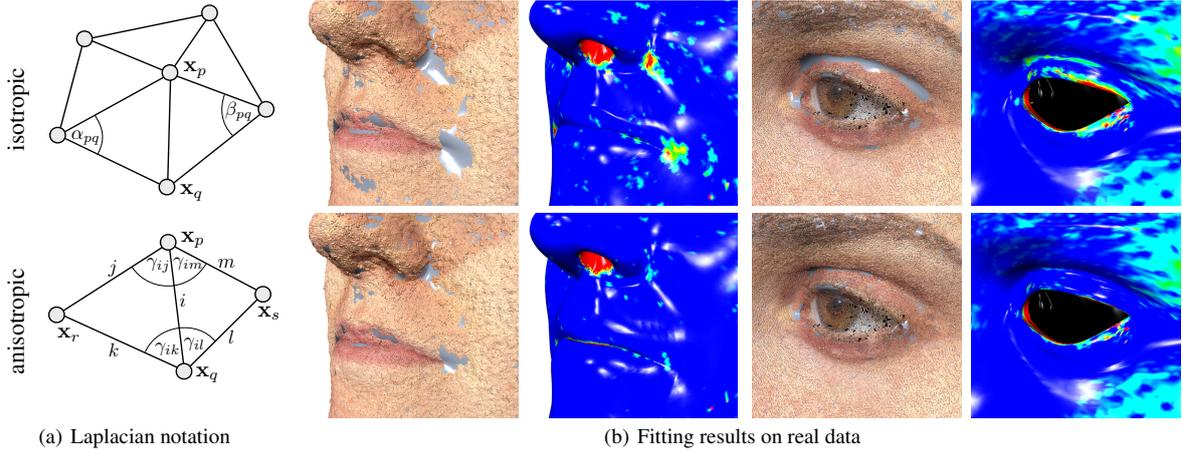
**Figure 4:** Notation for discrete Laplacians (a) and close-ups of fitting results (b) for isotropic (top) and anisotropic (bottom) bending energies. The anisotropic bending, using the Huber norm of edge Laplacians, yields more accurate fits of local facial features. The color coding visualizes the two-sided Hausdorff distance between the mesh and the point cloud.
