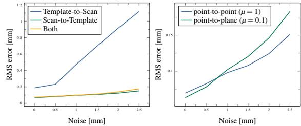
**Figure 2:** Comparison of correspondence directions (template-to-scan vs. scan-to-template, left) and correspondence distance (point-to-point vs. point-to-plane, right) on a high-resolution face scan with synthetically added noise (uniformly distributed, zero mean).
