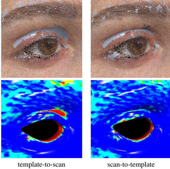
**Figure 3:** For high-resolution scanner data, our scan-to-template correspondences (right) yield more accurate reconstruction than the typically employed template-to-scan correspondences (left). The bottom row shows a color-coding of the two-sided Hausdorff distance of scan and template.
