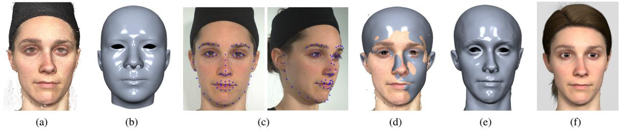
**Figure 1:** Template fitting pipeline: (a) Input point cloud, consisting of 1.4M sample points, (b) template mesh from FaceWarehouse with 12k vertices, (c) automatically detected facial features, (d) initial feature-based alignment, (e) final fit after non-rigid registration, (f) rendering with additional hair and eyes.
