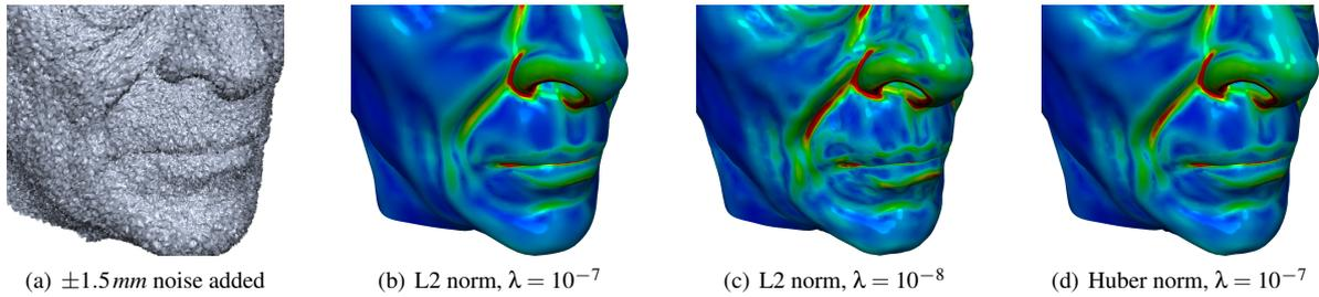
**Figure 5:** Comparison of isotropic and anisotropic bending on a synthetic model with added noise: The isotropic bending either does not fit the wrinkle well (b) or overfits the noisy input (c, see mouth region). The anisotropic model does not suffer from overfitting and reconstructs the wrinkle better. The RMS errors for (b), (c), and (d) are 0.36 mm, 0.43 mm, and 0.28 mm.
