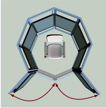
**Figure 2:** The OCTAVIS viewed from top. Two displays acts as door segments and allow to easily enter the system.
