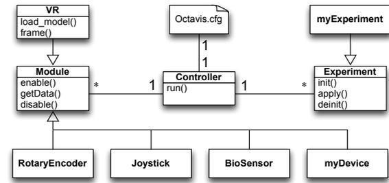
**Figure 7:** UML diagram of the main software architecture.
