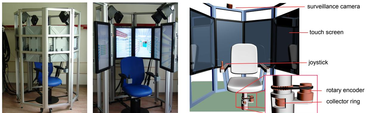
**Figure 1:** Two photographs (left) and a simplified illustration of our OCTAVIS VR-system. Eight screens, arranged in an octagon, provide a 360° panorama visualization of the virtual environment. Two door segments can be opened. Navigation in the VR is performed through a modified office chair, whose orientation determines the movement direction, and a “throttle joystick” in the armrest. Easy and natural interaction with objects is enabled through a simple touch screen interface.
