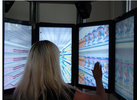
**Figure 5:** Photograph of a user navigating in the virtual supermarket and buying items via touch interface.
