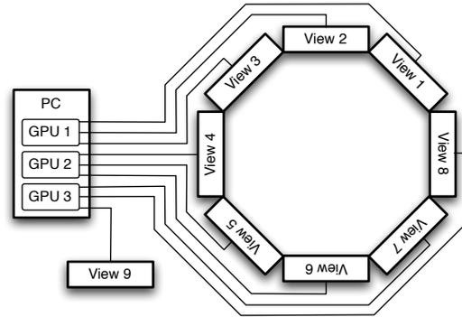
**Figure 3:** Schematic view of the hardware setup. One PC, equipped with three GPUs, drives the eight VR displays and an operator display.
